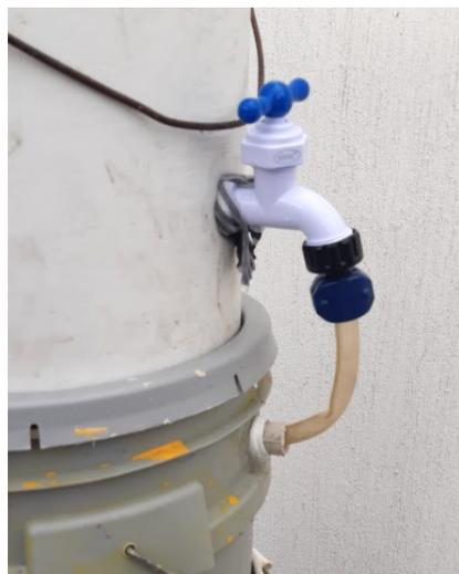
1. With a drill and the paddle bit, make the hole in the last bucket, where the coal will be included, put the faucet. Place the faucet, put a little Teflon on it to prevent leaks, secure it with a nut on its thread.
